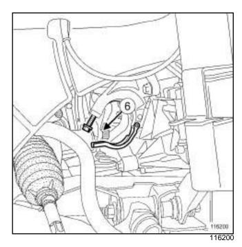
□ Remove the driveshaft relay bearing bracket mounting bolt (6).
