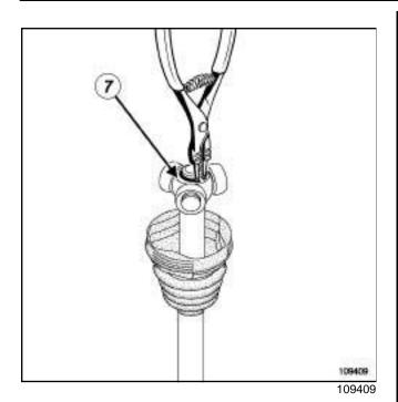
☐ Remove the lock ring (7) using the tool.
